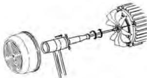
Check the that the direction of motor rotation corresponds with that indicated on the specification plate (the fan should rotate in a **CLOCKWISE DIRECTION**, when viewed from the rear of the motor. If the motor is three-phase and it is observed that it is rotating in the opposite direction, then two of the supply phases should be inverted at the protection panel.
