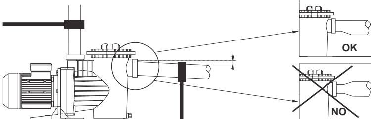
It is very important that both the suction and impulsion piping are independently supported and correctly fixed in place so that the pump does not have to support their weight nor the vibration produced by the water flow through them. In a situation where a long length of impulsion piping is used, we recommend the installation of a check valve to prevent the water hammer produced by the return of the water causing any damage when the pump stops.
